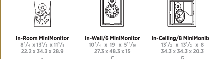
In-Room MiniMonitor 8 1/2" x 17 1/2" x 11 1/2" 22.2 x 34.3 x 28.9 In-Wall/6 MiniMonitor 10 1/2" x 19 x 5 7/8" 27.3 x 48.3 x 15 In-Ceiling/8 MiniMonitor 13 1/2" x 13 1/2" x 10 1/2" 34.3 x 34.3 x 20.3
